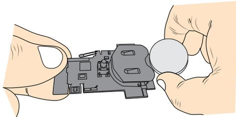
Replace the battery with a new **CR2450** battery.
