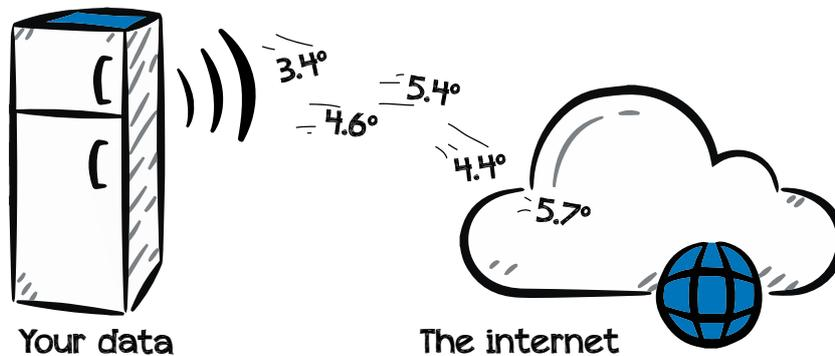
Clever Loggers are connected directly to the internet via a device called a gateway. The temperature in your fridge or freezer is recorded and saved to the internet every few minutes.
