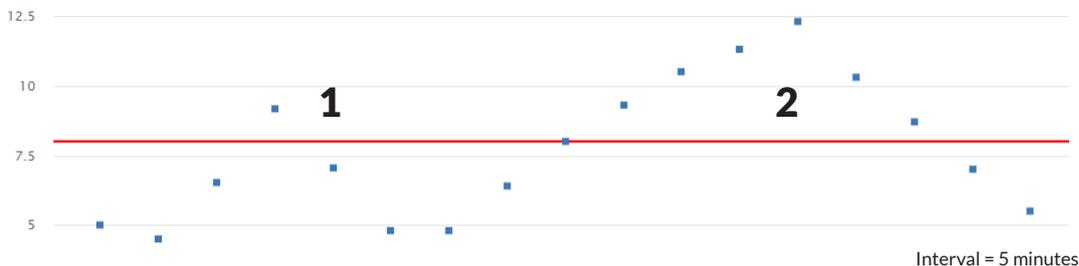
**Example: The delay is set to 15 minutes. The first spike (1) does not trigger the alarm because it lasts less than 15 minutes. The second spike (2) triggers an alarm because the temperature remains above the threshold for more than 15 minutes.**
