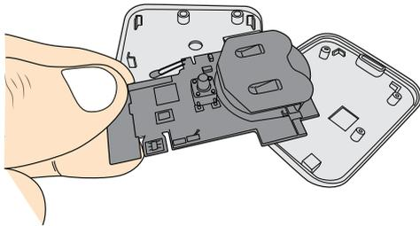
Remove the circuit board.
